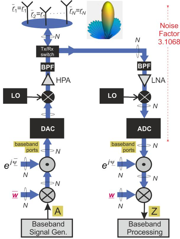
Figure 1: Monostatic Phased Array: System Modelling.
