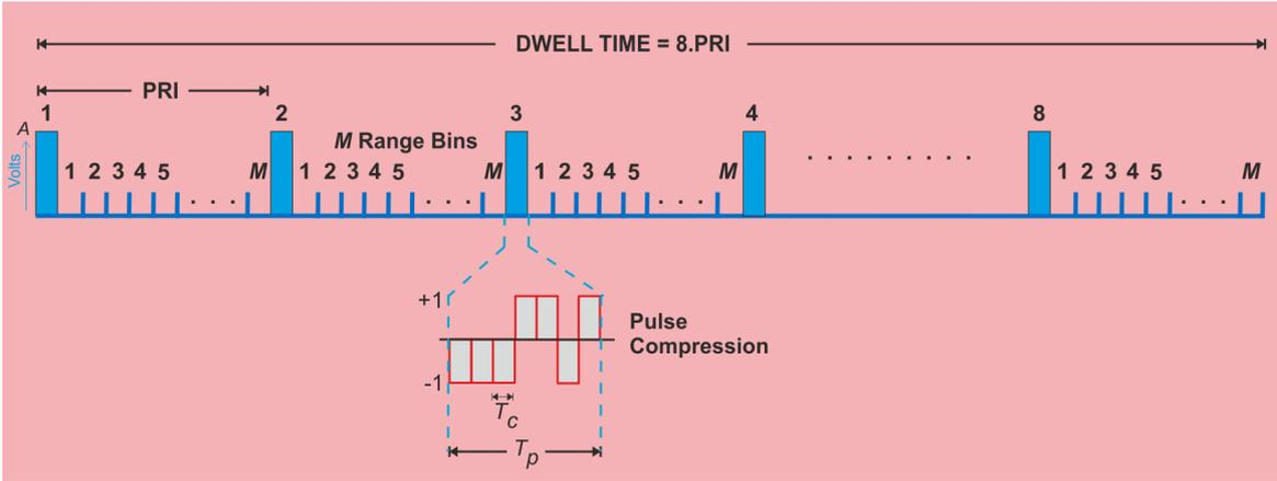
Figure 2: Transmitted Baseband Waveform (Single Direction).  $T_c = 28\text{ns}$ ,  $A = 1\text{kV}$ ,  $M = 199$ .
