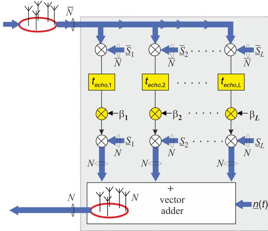
Figure 4: MIMO backscatter multi-target modelling
