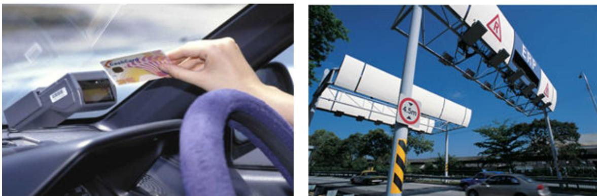
Figure 6.3: (a) In-vehicle Unit with CashCard and (b) ERP Gantry. (Source: [17])
